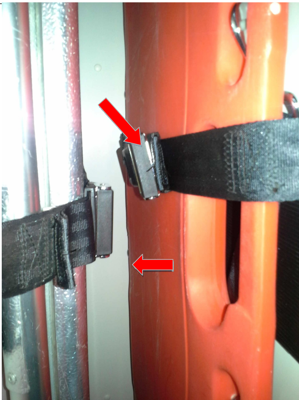
Fig. 66. Method of attaching the pick-up stretcher and orthopaedic board.
