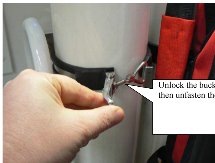
Figure 63: Method of unlocking the 10l oxygen cylinder rack.
