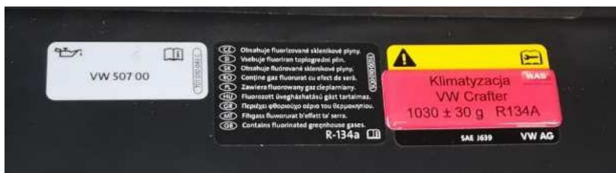
Fig. 23. Label in the engine compartment indicating the necessary amount of R134a gas.
