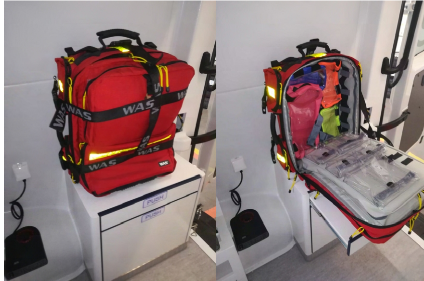
Figure 60: Cabinet with pull-out work surface in the right rear of the vehicle.
