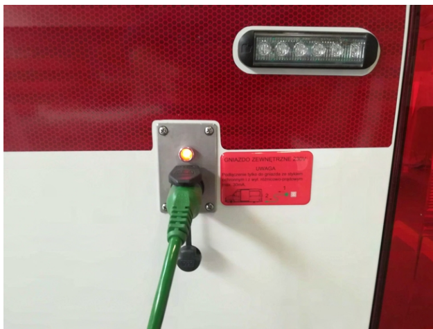
Fig. 67. Connection of external 230V power supply.
